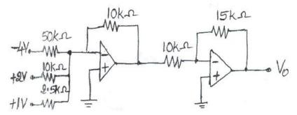
43. Find the output of the op-amp circuit shown in the figure below.
