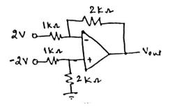
48. Determine V<sub>o</sub> for the circuit shown below.
