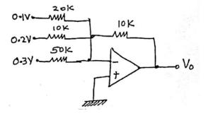
49. For the circuit shown in the figure, calculate the output voltage.
