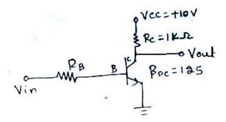
9. The transistor in common emitter configuration is shown in figure, with  $R_C = 10 \text{ k}\Omega$  and  $\beta_{dc} = 200$ . Determine (i)  $V_{CE}$  at  $V_{in} = 0$  (ii)  $I_{B(min)}$  to saturate the collector current (iii)  $R_{B(max)}$  when  $V_{in} = 5 \text{ V. } V_{CE(sat)}$  can be neglected. (Jan '19 – 4M)
